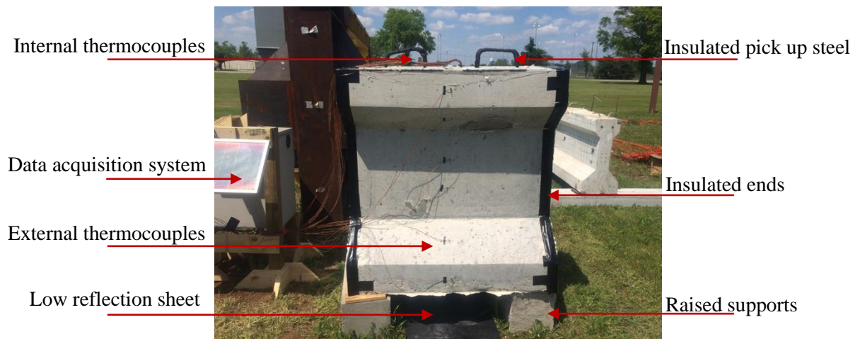
Figure 3.7 - Fully instrumented Type IV girder segment – Norman, OK
