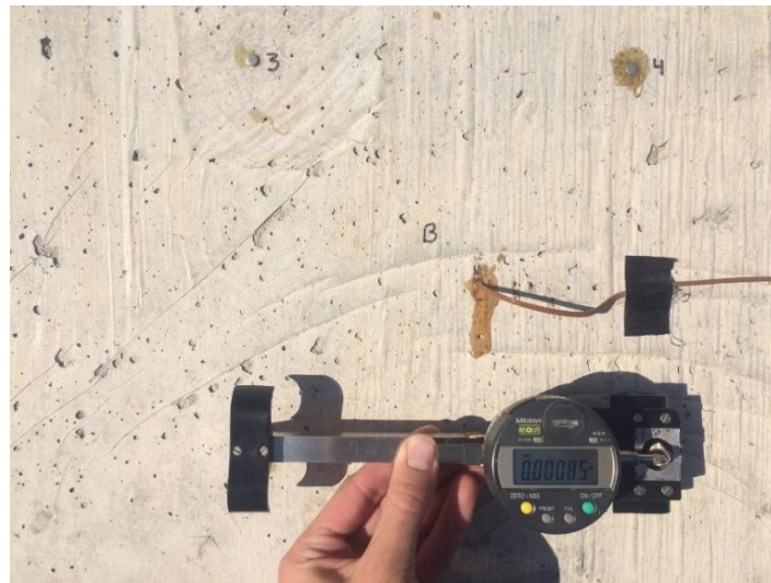
Figure 3.4 – Expansion/strain measurement with DEMEC gauge
